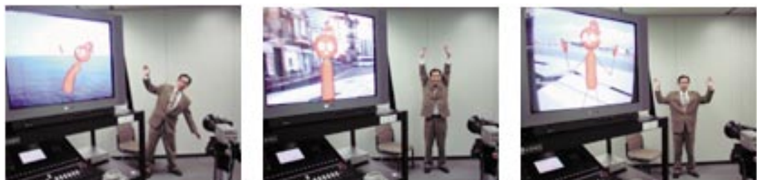
Figure 11. Scenes from the Networked Theater. A CCD camera captures the person’s motion and reproduces it in the red character displayed on the screen.
