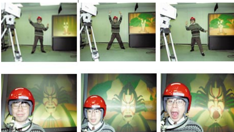
Figure 8. Scenes of the Virtual Kabuki system. The infrared camera observes the person, and the estimated postures are reproduced in the Kabuki actor's model displayed in the projector screen (top row). The camera fixed to the helmet observes the face, and the estimated facial expressions are reproduced in the Kabuki actor's face model (bottom row).
